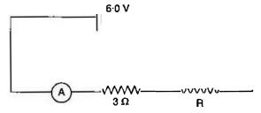
When the circuit is switched on, the ammeter reads 0.5 A.
